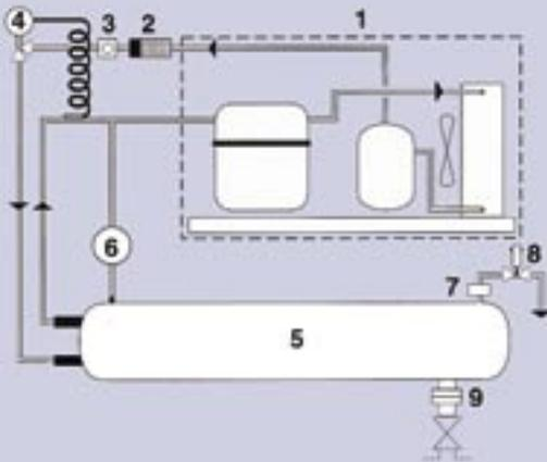
1. Condensing unit 2. Filter 3. Sight glass 4. Thermostatic expansion valve 5. Heat exchanger 6. LP and HP pressure controller 7. Calibrated restriction 8. Purging solenoid valve 9. Flanged connection
